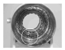
10. Looking from the opposite end of the housing (1) you can see if your timing marks are lining up. When they do, tap the piston (3) in until the gear teeth mesh together. Tap the piston into the housing the rest of the way until it bottoms out.
