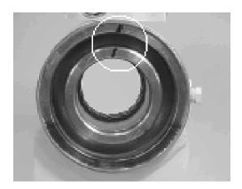
9. Looking from the angle shown, rotate the piston (3) until the marks you put on the piston and the housing (1) during disassembly line up as shown. Using a rubber mallet, tap the piston into the housing up to the point where the gear teeth meet.
