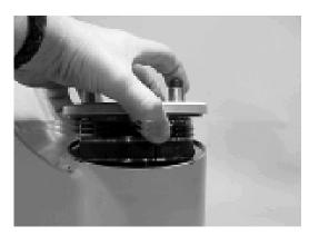
**6.** Remove the end cap (4) and set aside for later inspection.
