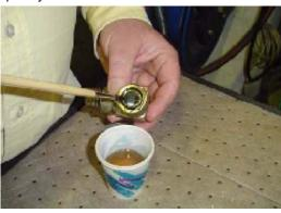
**3.** Turn the o-ring on the other side of the fitting and repeat the previous step, ensuring the entire o-ring is coated with hydraulic oil.
