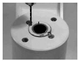
2. Using a 1/8" (3.18mm) drill bit, drill a hole in the center of each lock pin to a depth of approximately 3/16" (4.76mm).
