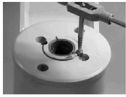
3. Remove the lock pins using an "Easy Out" (a size #2 is shown). If the pin will not come out with the "Easy Out", use 5/16" drill bit to a depth of 1/2" (12.7mm)todrill out the entire pin.
