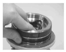
**16.** Install the O-ring (204) and back-up ring (207) into the inner seal groove on the end cap (4).
