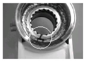
11. Before removing the piston (3), mark the housing (1) ring gear in relation to the piston O.D. gear. There should now be timing marks on the housing (1) ring gear, the piston (3) and the shaft (2).
