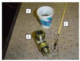
1. Hold the fitting in one hand while using the brush with the other hand to dip into the container. Remove excess hydraulic oil from the brush so an even film of oil is applied on the o-ring.
