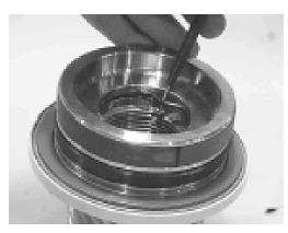
**14.** Remove the o-ring (204) and backup ring (207) from end cap (4) and set aside for inspection.
