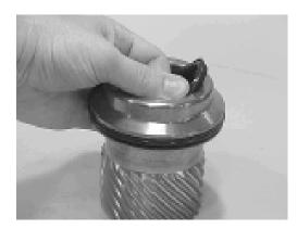
6. Install the inner T-seal (200) into the piston (3) using a circular motion. Install the outer T-seal (202) by stretching it around the groove in a circular motion. Each T-seal has 2 back-up rings (see drawing for orientation).
