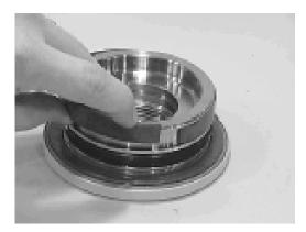
Install the wear guide (302) on the end cap (4) and shaft (2).
