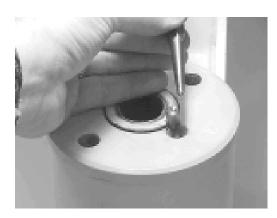
19. Remove the piston O.D. seal (202).
