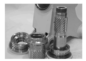
Clean all parts in a solvent tank and dry with compressed air prior to inspecting. Carefully inspect all critical areas for any surface finish abnormalities: Seal grooves, bearing grooves, thrust surfaces, rod surface, housing bore and gear teeth.
