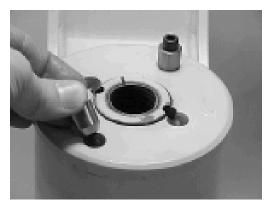
**4.** Install the end cap (4) removal tools provided with the Helac seal kit.
