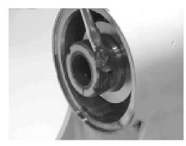
**15.** Coat the threads on the end of the shaft with antiseize grease to prevent galling.
