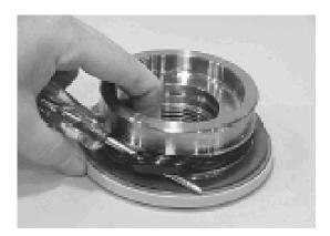
Using a seal tool install the main pressure seal (205) onto shaft (2) and end cap (4). Use the seal tool in a circular motion.
