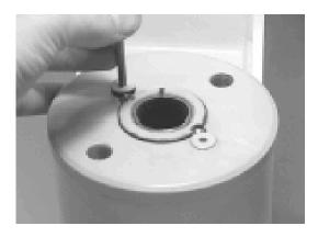
**20.** Insert the set screws (113) over the lock pins. Tighten them to 25 in. lbs. (2.825 Nm).
