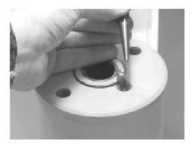
**19.** Place the lock pins (109) provided in the Helac seal kit in the holes with the dimple side up. Then, using a punch, tap the lock pins to the bottom of the hole.
