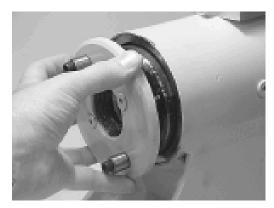
17. Thread the end cap (4) onto the shaft (2) end. Make sure the wear guide stays in place on the end cap as it is threaded into the housing (1).
