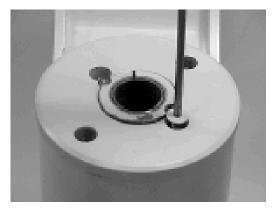
Remove the cap screws (113) over end cap lock pins (109).
