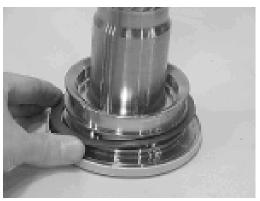
2. Install the thrust washer (304) onto shaft (2) and end cap (4).
